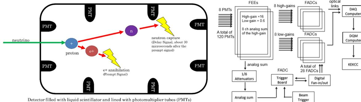
Fig1: A diagram of the JSNS<sup>2</sup> detector and DAQ system as seen in [4]. Neutrinos that enter the detector may interact via IBD which produces two flashes of light that are recorded by the PMTs and sent to the DAQ system. The DAQ system processes these analog signals and turns them into digital data.
