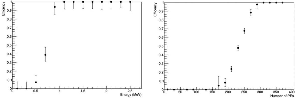
Fig3: (left) The efficiency of the trigger is plotted against the energy of the event for a simulation of 500 e<sup>-</sup> with 0 to 2.5MeV. (right) The efficiency of the trigger is plotted against the number of photoelectrons produced by each event for 1MeV e<sup>-</sup>. In both cases the e<sup>-</sup> were placed randomly within the inner detector volume. The behavior seen here indicates that the trigger simulation is behaving as expected.
