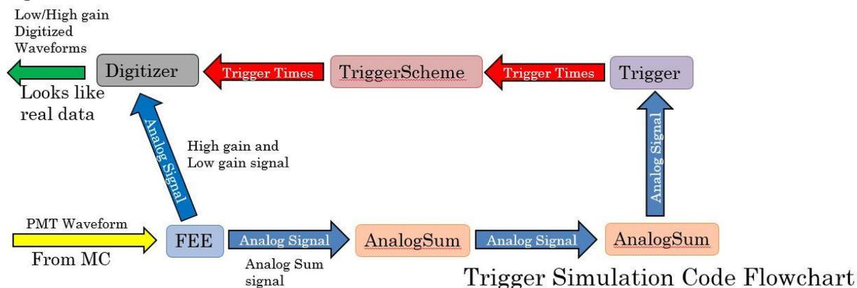
Fig2: A flowchart of the code I added to the DAQ simulation meant to simulate the JSNS<sup>2</sup> trigger simulation. Most of the code of the added code is contained in three classes, `AnalogSum`, which simulates analog sum circuitry, `Trigger`, which finds above threshold times, and `TriggerScheme`, which build the various veto schemes that select trigger times that meet certain criteria.
