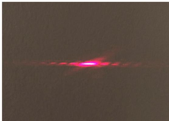
Figure 1 An image of the diffraction pattern created by the handmade single slit slide.
