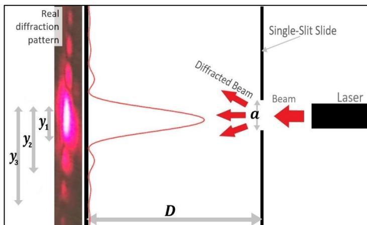
Figure 3. A diagram I created which shows the proper experimental setup for the single slit diffraction activity.
