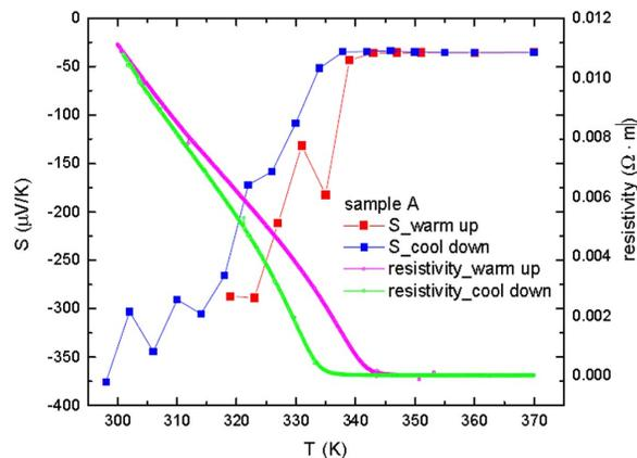
Figure 2: Resistivity and thermopower from the test of the high-temperature probe. Both show the MIT at around 70°C. The thermopower measurement suffers due to the high thermal noise of the system. Graph by Lu Chen
