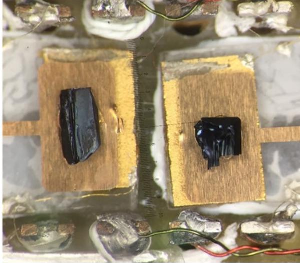
Figure 4: The set-up for the samarium hexaboride test. The left sample was roughened by the polishing process and is therefore duller.
