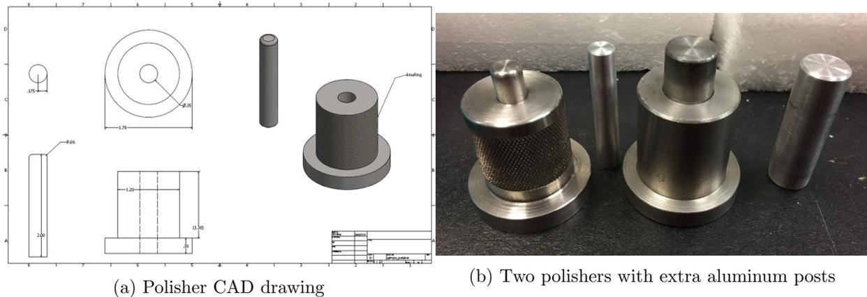
Figure 3: The initial CAD drawing of the polisher and the final result. The polisher on the right is the newer design.
