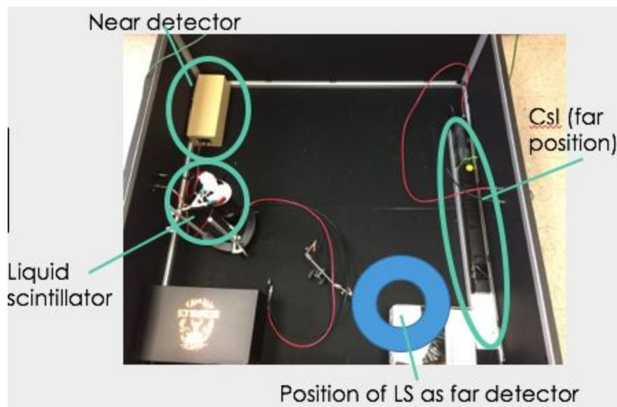
Figure 2: Experimental setup with labeled near and far detectors. In this image, the CsI crystal was acting as the far detector, so if the liquid scintillator was acting as the far detector, it would be placed where the thick blue circle indicates.
