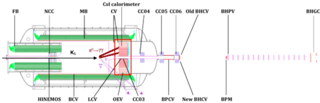
Figure 1: Side view of the KOTO detector, with a  $K_L^0 \rightarrow \pi^0 \nu \bar{\nu}$  decay being shown inside the detector. You can see the different directions of pion and resulting photons in comparison to the direction of the resulting neutrinos.
