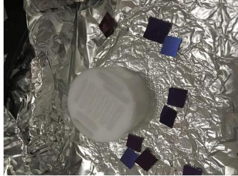
Figure 2. Specialized 3-D printed part used for cleaning substrates
