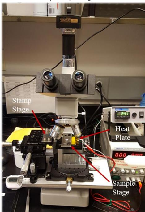
Figure 3. Microscope set-up for sample transfer.
