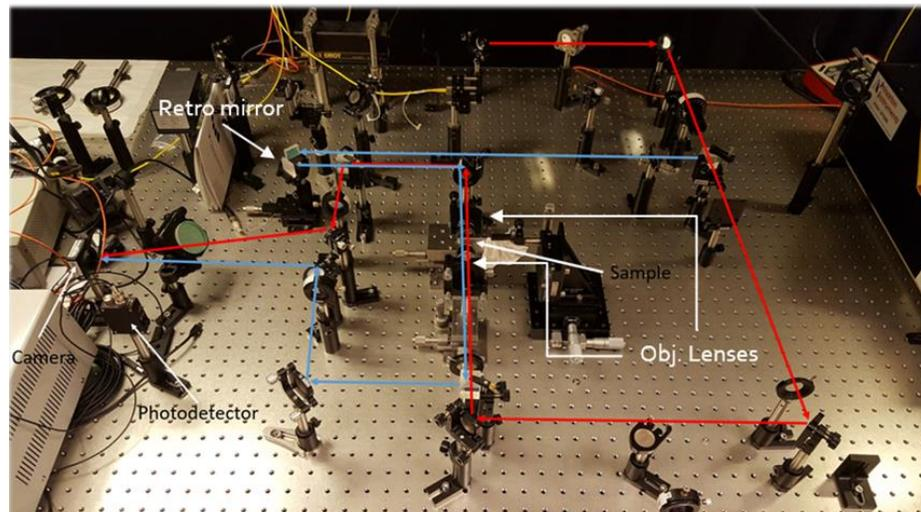
Figure 5. CPA experimental set-up, red and blue arrows indicating the path of the beams leading to a camera or photodetector.
