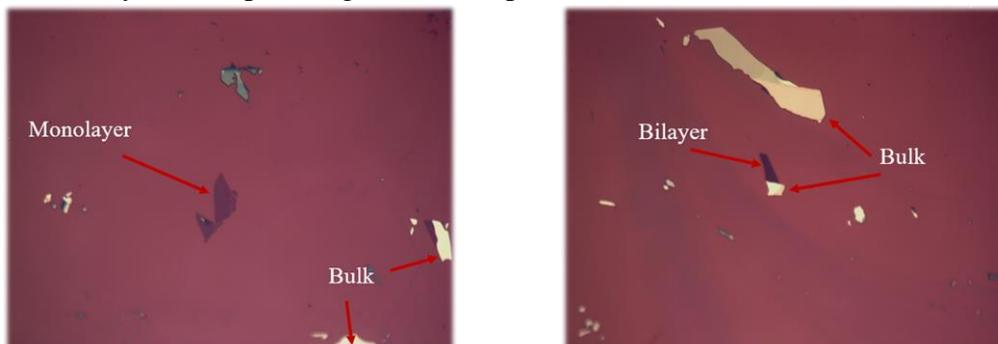
Figure 2. Monolayer and bilayer samples (respectively) of  $\text{WSe}_2$  on a Si substrate with bulk samples for reference.
