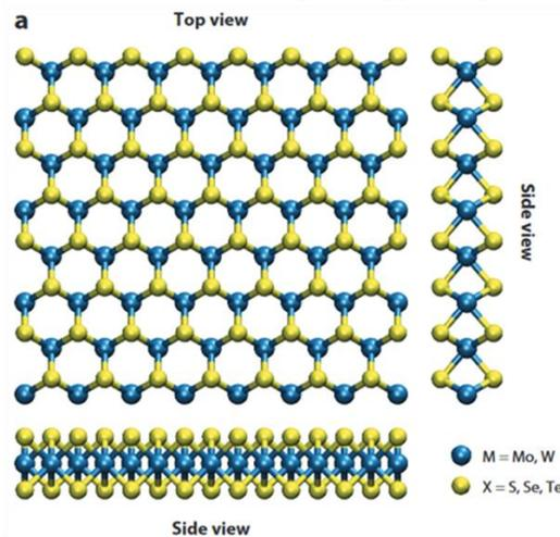
Figure 1. Top and side view of TMD structure courtesy of [2].
