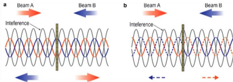
Figure 4. *a)* Destructive wave interference and *b)* constructive wave interference. Image courtesy of [6].
