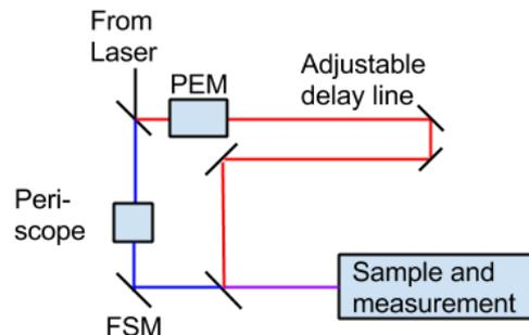
FIG. 1: A slightly inaccurate simplification of the setup. The FSM is the Fast Steering Mirror, used to control the distance of the pump beam (red) from the probe beam (blue). The PEM is a photoelastic modulator, which turns the linearly polarized light into circularly polarized light to pump spins into the sample.
