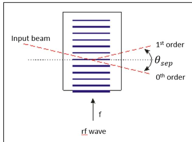
Figure 1: Schematic of an acousto-optic modulator
