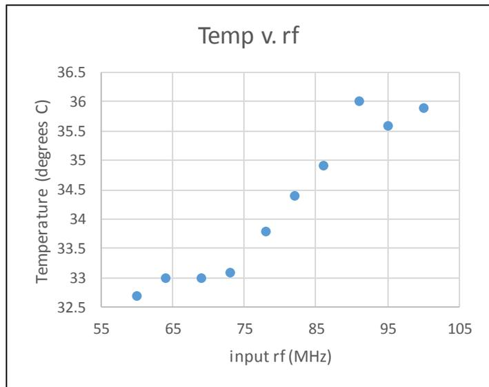
Figure 4: variation in AOM temperature as function of rf frequency
